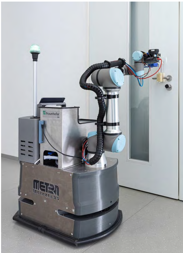
Figure 3.5: Using its cleaning brushes, DeKonBot 2 removes coarse dirt from door handles and comprehensively applies the disinfection fluid. Image credit: Fraunhofer IPA.
