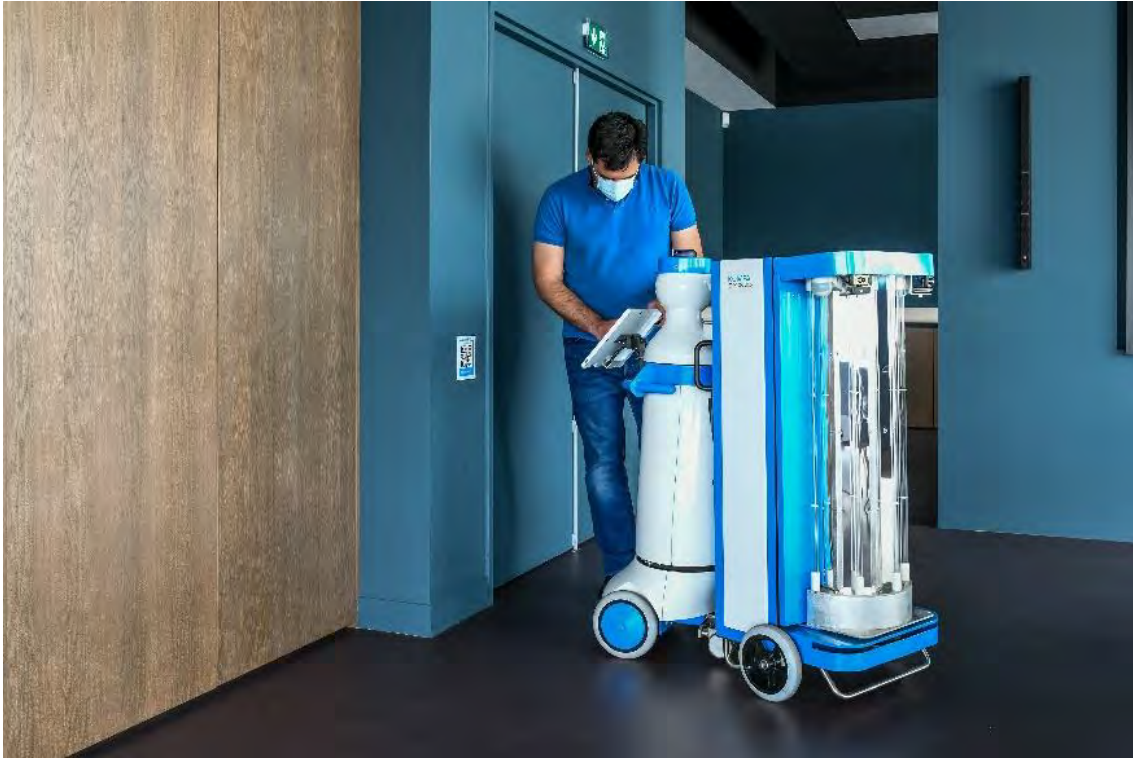
Figure 3.3: Since March 2021, the French company Kompaï has also been offering a disinfection robot with UV-C light. Image credit: Kompaï Robotics.
