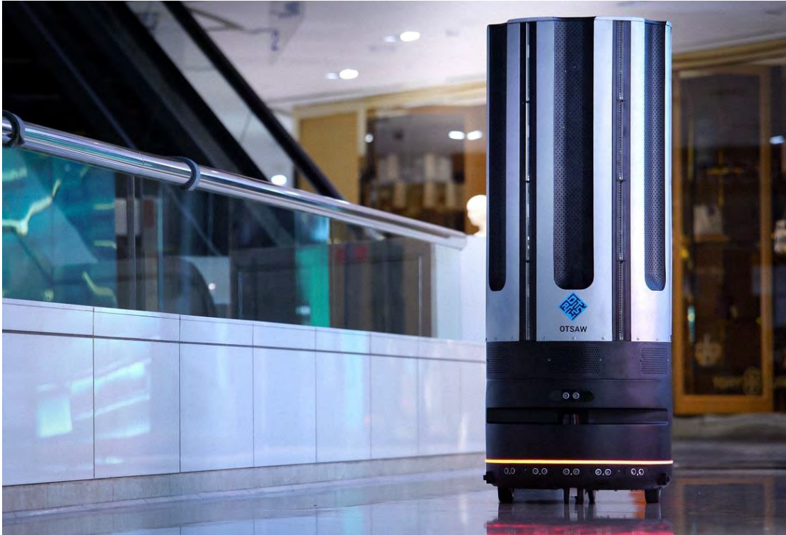
Figure 3.4: O-RX is a UV-C LED autonomous disinfecting robot with a disinfection rate of 99.999% at 2.5 meters. Image credit: OTSAW Digital.
