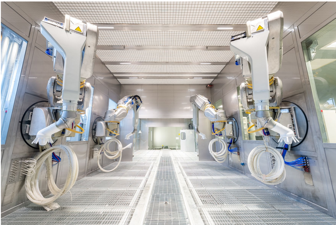
Figure 4: Media hoses and signal lines are routed through the central axis of the robot to the atomizer
