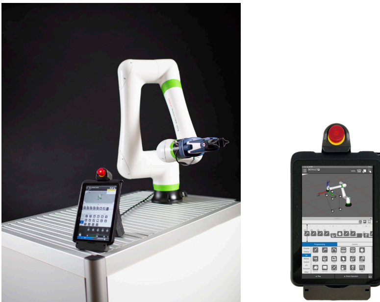
Figure1: FANUC CRX (“FANUC timeline programming” is shown on the screen of TP)
