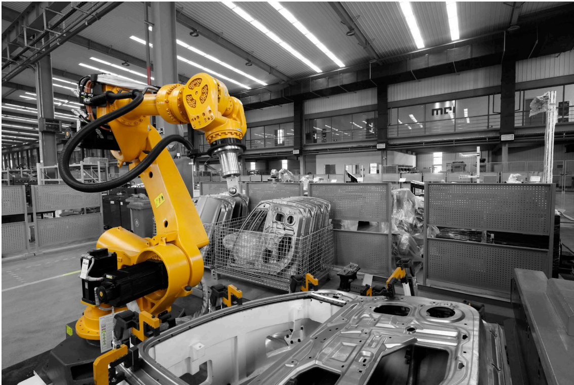
Figure 3: Beyond the use of robots in car body manufacturing, manufacturers will need to seek out new areas of application in the future. Image credit: Estun Robotics.
