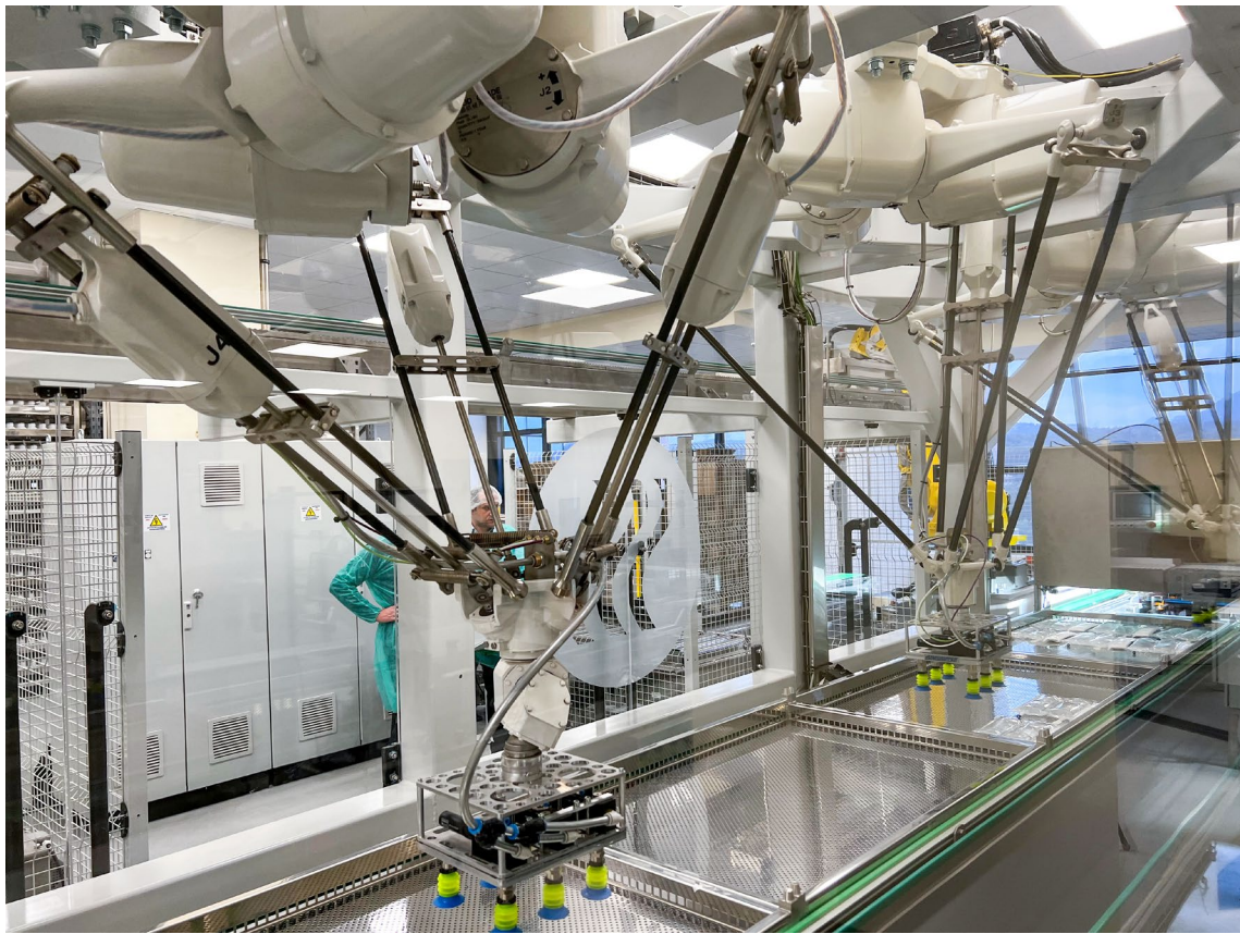
Figure 1: Robots handling plastic bags for sterilisation. Image credit: FANUC.
