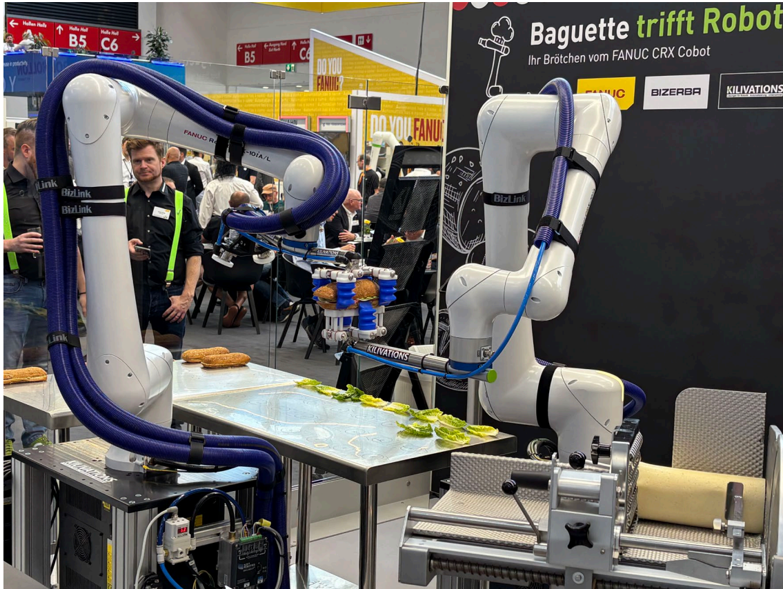
Figure 2: Cobots place cold cuts on baguettes. Image credit: FANUC.
