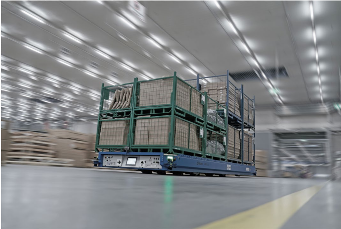
Figure 5: AutoBox, moving pallets indoor, Stäubli WFT
