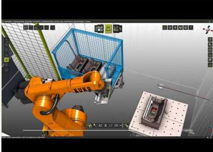
*Digital twin of a KUKA machine tending robot*
